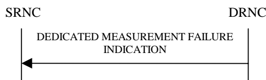
Figure 24: Dedicated Measurement Failure procedure, Successful Operation
