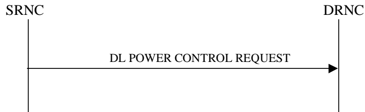
Figure 25: Downlink Power Control procedure, Successful Operation
