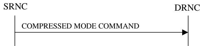
Figure 26: Compressed Mode Command procedure, Successful Operation
