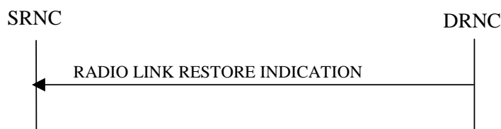
Figure 19: RL Restoration procedure, Successful Operation
