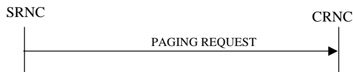
Figure 4: Paging procedure, Successful Operation
