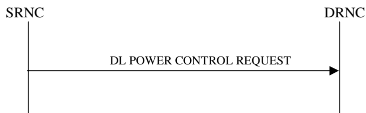
Figure 25: Downlink Power Control procedure, Successful Operation
