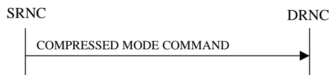
Figure 26: Compressed Mode Command procedure, Successful Operation
