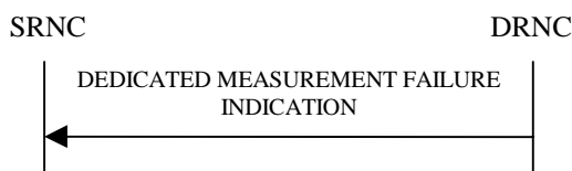
Figure 24: Dedicated Measurement Failure procedure, Successful Operation
