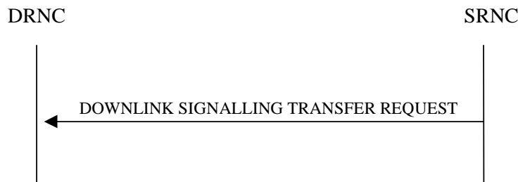
Figure 2: Downlink Signalling Transfer procedure, Successful Operation
