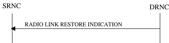
Figure 19: Radio Link Restoration procedure, Successful Operation
