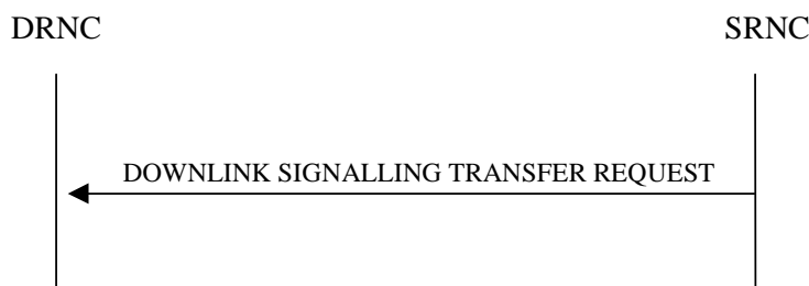
Figure 2: Downlink Signalling Transfer procedure, Successful Operation
