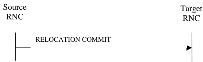
Figure 3: Relocation Commit procedure, Successful Operation
