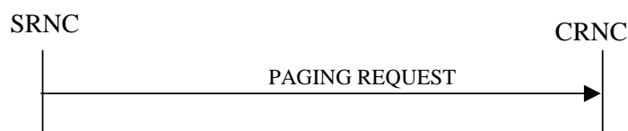
Figure 4: Paging procedure, Successful Operation
