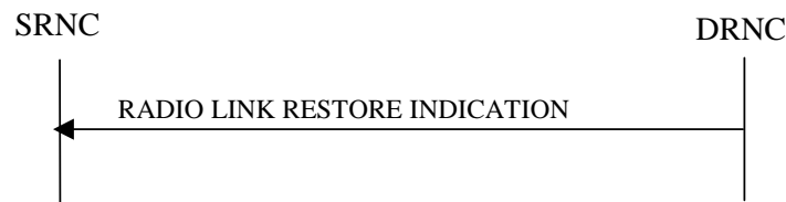
Figure 19: RL Restoration procedure, Successful Operation
