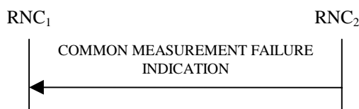
Figure 30E: Common Measurement Failure procedure, Successful Operation
