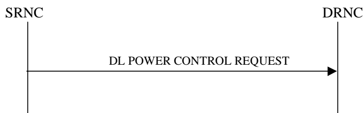
Figure 25: Downlink Power Control procedure, Successful Operation
