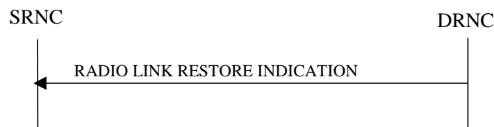
Figure 19: Radio Link Restoration procedure, Successful Operation
