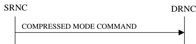
Figure 26: Compressed Mode Command procedure, Successful Operation
