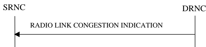
Figure 26C: Radio Link Congestion procedure, Successful Operation
