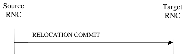
Figure 3: Relocation Commit procedure, Successful Operation
