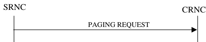
Figure 4: Paging procedure, Successful Operation
