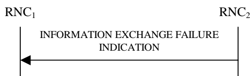
Figure 30J: Information Exchange Failure procedure, Successful Operation
