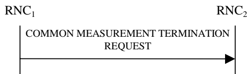
Figure 30D: Common Measurement Termination procedure, Successful Operation
