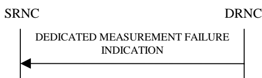
Figure 24: Dedicated Measurement Failure procedure, Successful Operation
