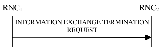
Figure 30I: Information Exchange Termination procedure, Successful Operation
