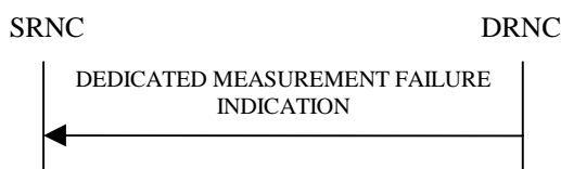
Figure 24: Dedicated Measurement Failure procedure, Successful Operation
