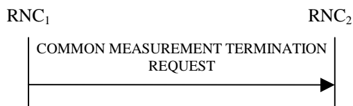
Figure 30D: Common Measurement Termination procedure, Successful Operation
