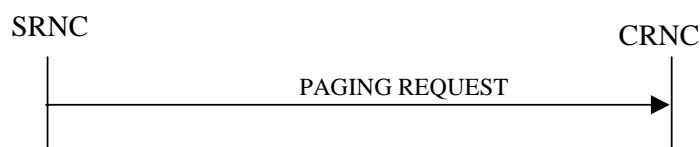
Figure 4: Paging procedure, Successful Operation
