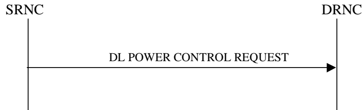
Figure 25: Downlink Power Control procedure, Successful Operation
