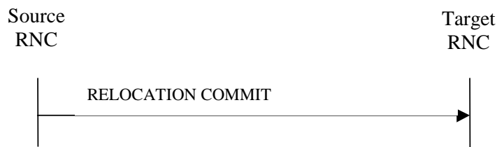
Figure 3: Relocation Commit procedure, Successful Operation
