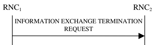
Figure 30I: Information Exchange Termination procedure, Successful Operation
