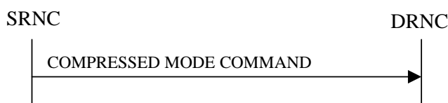
Figure 26: Compressed Mode Command procedure, Successful Operation
