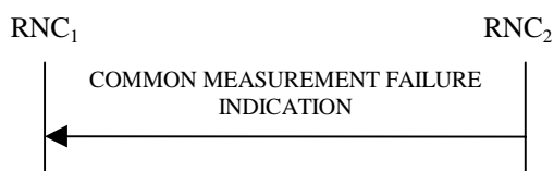
Figure 30E: Common Measurement Failure procedure, Successful Operation
