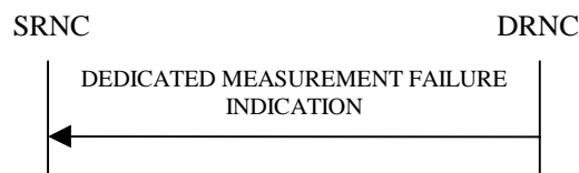
Figure 24: Dedicated Measurement Failure procedure, Successful Operation
