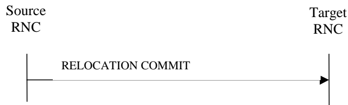
Figure 3: Relocation Commit procedure, Successful Operation
