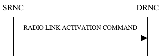
Figure 26D: Radio Link Activation procedure
