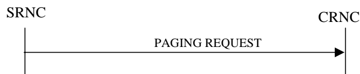
Figure 4: Paging procedure, Successful Operation
