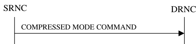
Figure 26: Compressed Mode Command procedure, Successful Operation
