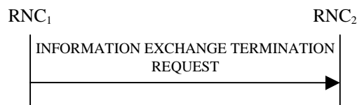
Figure 30I: Information Exchange Termination procedure, Successful Operation
