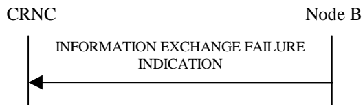
Figure 30J: Information Exchange Failure procedure, Successful Operation
