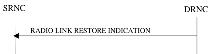
Figure 19: Radio Link Restoration procedure, Successful Operation
