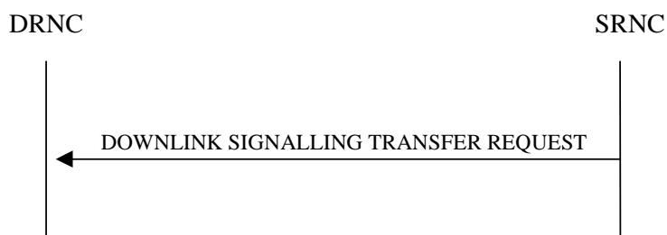
Figure 2: Downlink Signalling Transfer procedure, Successful Operation
