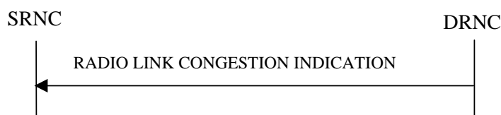
Figure 26C: Radio Link Congestion procedure, Successful Operation
