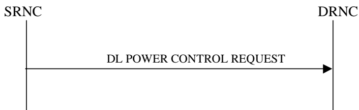
Figure 25: Downlink Power Control procedure, Successful Operation
