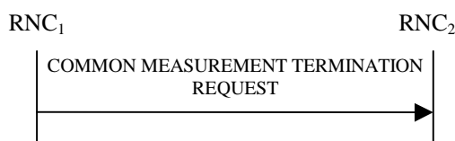
Figure 30D: Common Measurement Termination procedure, Successful Operation
