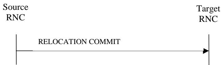
Figure 3: Relocation Commit procedure, Successful Operation
