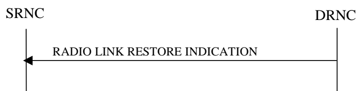
Figure 19: Radio Link Restoration procedure, Successful Operation
