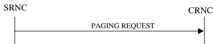
Figure 4: Paging procedure, Successful Operation
