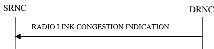
Figure 26C: Radio Link Congestion procedure, Successful Operation
