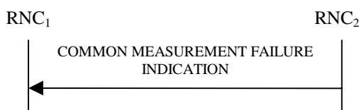
Figure 30E: Common Measurement Failure procedure, Successful Operation
