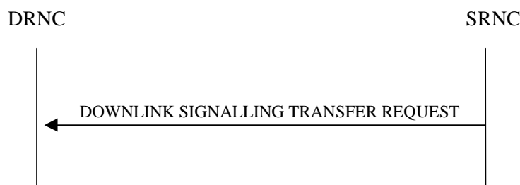
Figure 2: Downlink Signalling Transfer procedure, Successful Operation
