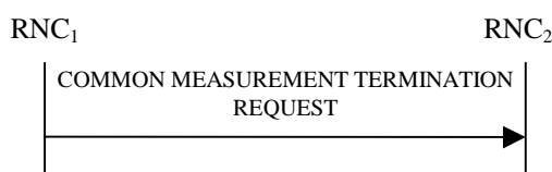
Figure 30D: Common Measurement Termination procedure, Successful Operation
