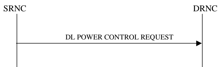
Figure 25: Downlink Power Control procedure, Successful Operation
