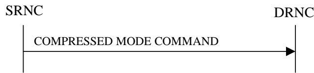
Figure 26: Compressed Mode Command procedure, Successful Operation
