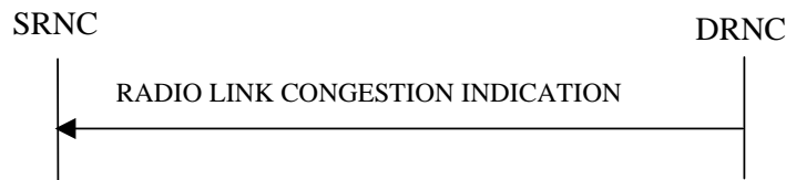
Figure 26C: Radio Link Congestion procedure, Successful Operation
