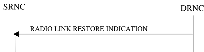
Figure 19: Radio Link Restoration procedure, Successful Operation
