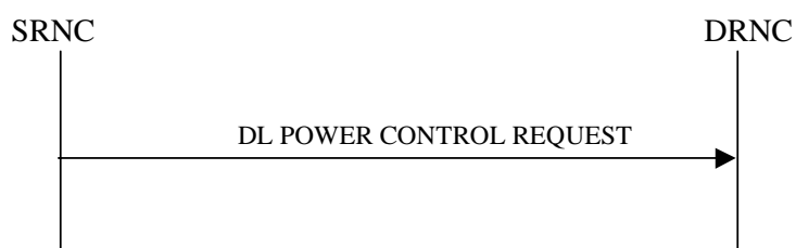
Figure 25: Downlink Power Control procedure, Successful Operation
