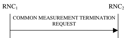
Figure 30D: Common Measurement Termination procedure, Successful Operation
