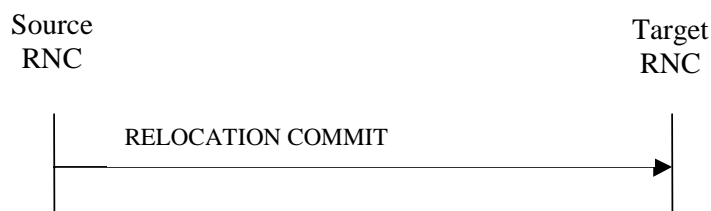
Figure 3: Relocation Commit procedure, Successful Operation
