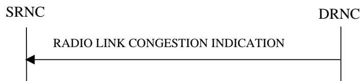
Figure 26C: Radio Link Congestion procedure, Successful Operation
