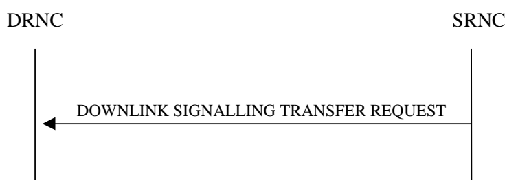
Figure 2: Downlink Signalling Transfer procedure, Successful Operation
