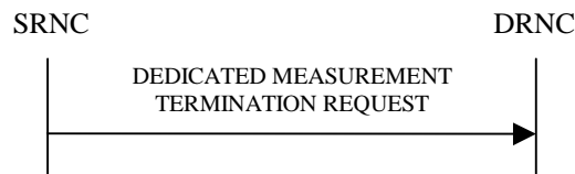
Figure 23: Dedicated Measurement Termination procedure, Successful Operation
