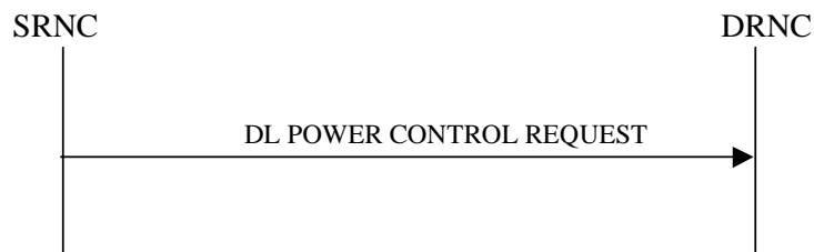
Figure 25: Downlink Power Control procedure, Successful Operation
