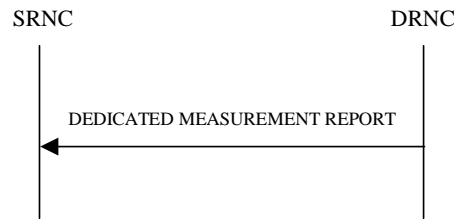
Figure 22: Dedicated Measurement Reporting procedure, Successful Operation
