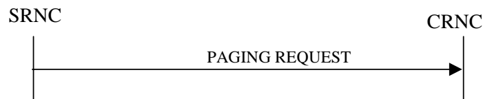
Figure 4: Paging procedure, Successful Operation
