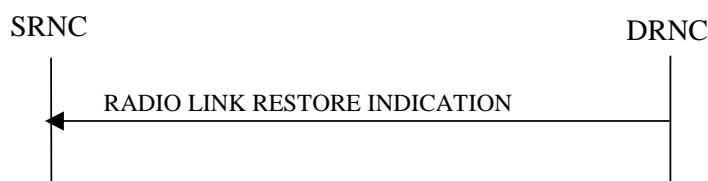
Figure 19: Radio Link Restoration procedure, Successful Operation
