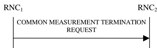
Figure 30D: Common Measurement Termination procedure, Successful Operation
