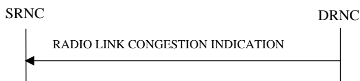
Figure 26C: Radio Link Congestion procedure, Successful Operation
