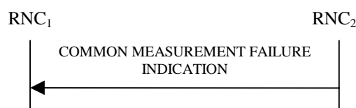
Figure 30E: Common Measurement Failure procedure, Successful Operation
