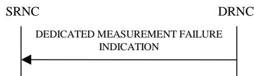
Figure 24: Dedicated Measurement Failure procedure, Successful Operation
