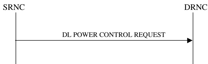
Figure 25: Downlink Power Control procedure, Successful Operation
