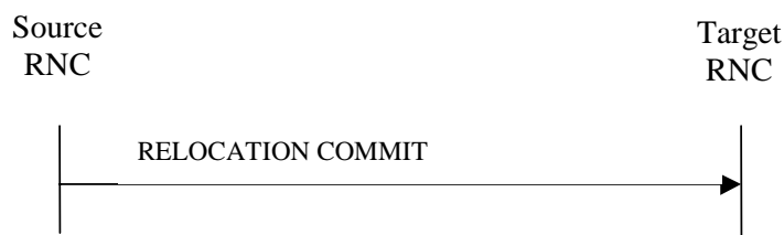
Figure 3: Relocation Commit procedure, Successful Operation
