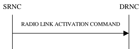
Figure 26D: Radio Link Activation procedure
