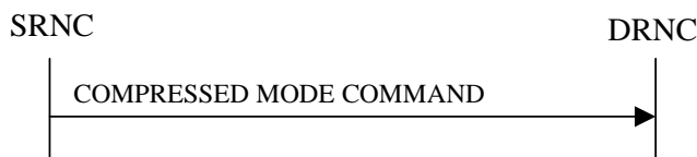
Figure 26: Compressed Mode Command procedure, Successful Operation
