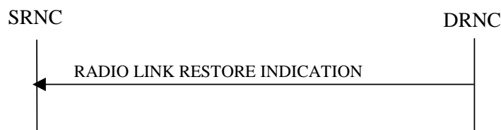
Figure 19: Radio Link Restoration procedure, Successful Operation
