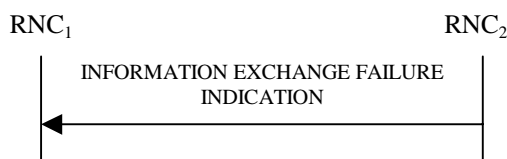
Figure 30J: Information Exchange Failure procedure, Successful Operation
