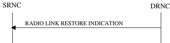
Figure 19: Radio Link Restoration procedure, Successful Operation
