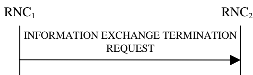
Figure 30I: Information Exchange Termination procedure, Successful Operation
