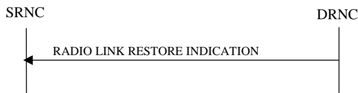
Figure 19: Radio Link Restoration procedure, Successful Operation
