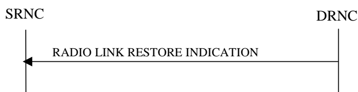
Figure 19: Radio Link Restoration procedure, Successful Operation
