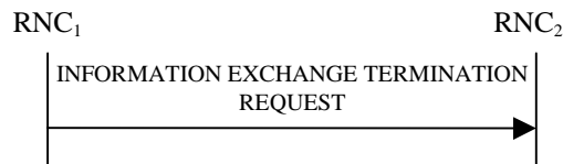
Figure 30I: Information Exchange Termination procedure, Successful Operation
