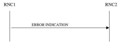
Figure 30: Error Indication procedure, Successful Operation
