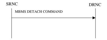
Figure 32: MBMS Detach procedure, Successful Operation
