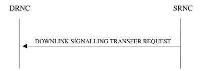
Figure 2: Downlink Signalling Transfer procedure, Successful Operation
