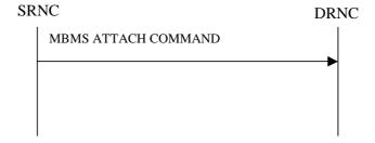
Figure 31: MBMS Attach procedure, Successful Operation
