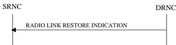
Figure 19: Radio Link Restoration procedure, Successful Operation
