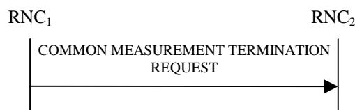
Figure 30D: Common Measurement Termination procedure, Successful Operation
