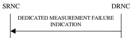
Figure 24: Dedicated Measurement Failure procedure, Successful Operation
