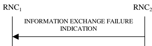
Figure 30J: Information Exchange Failure procedure, Successful Operation
