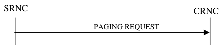
Figure 4: Paging procedure, Successful Operation
