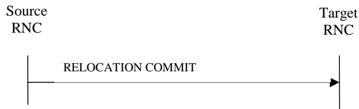
Figure 3: Relocation Commit procedure, Successful Operation
