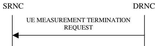
Figure 26I: UE Measurement Termination procedure, Successful Operation
