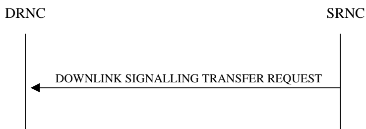
Figure 2: Downlink Signalling Transfer procedure, Successful Operation
