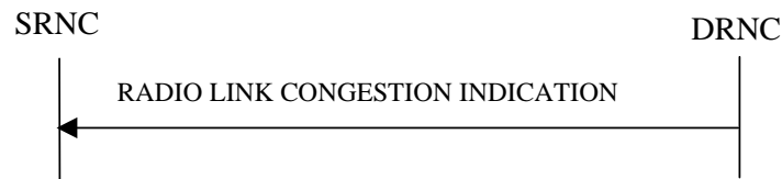
Figure 26C: Radio Link Congestion procedure, Successful Operation
