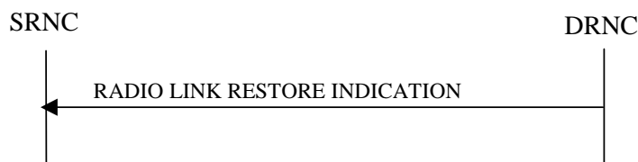
Figure 19: Radio Link Restoration procedure, Successful Operation
