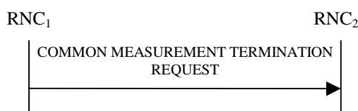
Figure 30D: Common Measurement Termination procedure, Successful Operation
