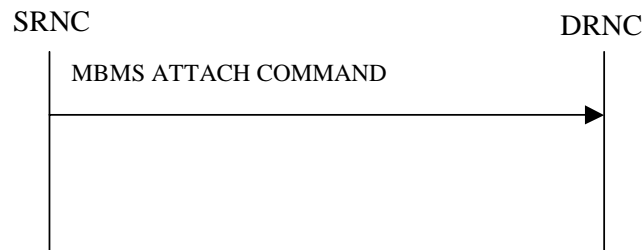
Figure 31: MBMS Attach procedure, Successful Operation
