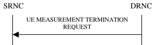
Figure 26I: UE Measurement Termination procedure, Successful Operation
