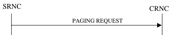
Figure 4: Paging procedure, Successful Operation
