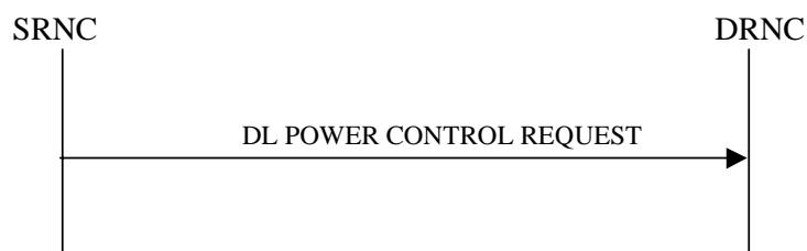
Figure 25: Downlink Power Control procedure, Successful Operation
