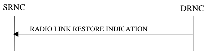
Figure 19: Radio Link Restoration procedure, Successful Operation
