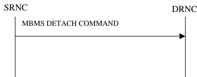
Figure 32: MBMS Detach procedure, Successful Operation
