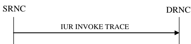
Figure 26K: Iur Invoke Trace procedure, Successful Operation
