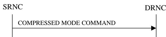
Figure 26: Compressed Mode Command procedure, Successful Operation
