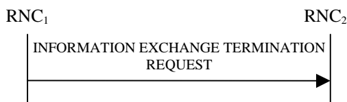
Figure 30I: Information Exchange Termination procedure, Successful Operation
