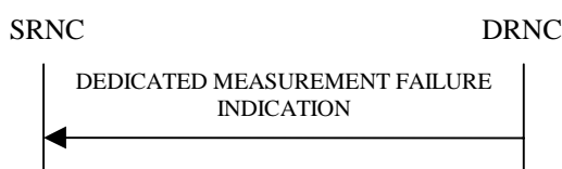
Figure 24: Dedicated Measurement Failure procedure, Successful Operation
