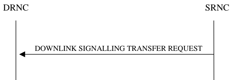
Figure 2: Downlink Signalling Transfer procedure, Successful Operation
