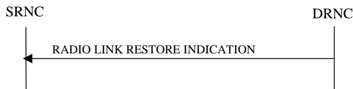
Figure 19: Radio Link Restoration procedure, Successful Operation
