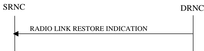
Figure 19: Radio Link Restoration procedure, Successful Operation
