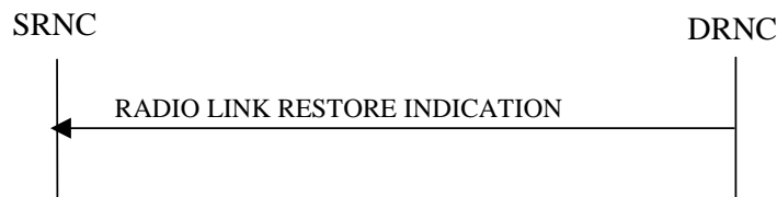
Figure 19: Radio Link Restoration procedure, Successful Operation
