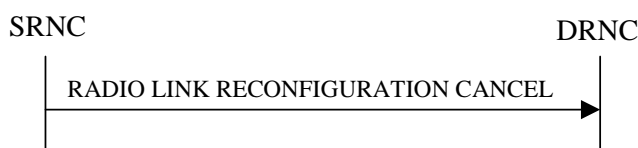
Figure 13: Synchronised Radio Link Reconfiguration Cancellation procedure, Successful Operation
