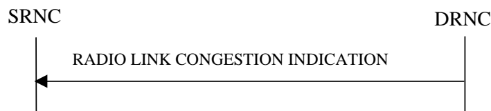
Figure 26C: Radio Link Congestion procedure, Successful Operation
