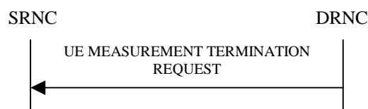
Figure 26I: UE Measurement Termination procedure, Successful Operation
