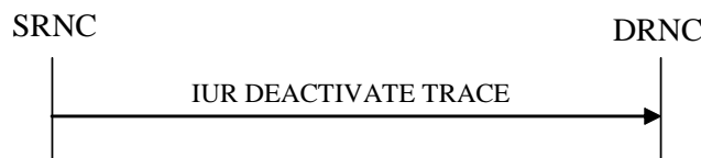
Figure 26L: Iur Deactivate Trace procedure, Successful Operation
