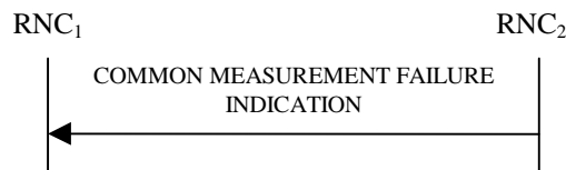
Figure 30E: Common Measurement Failure procedure, Successful Operation
