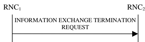
Figure 30I: Information Exchange Termination procedure, Successful Operation
