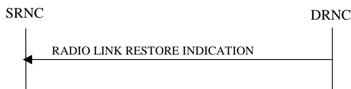
Figure 19: Radio Link Restoration procedure, Successful Operation
