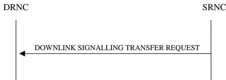
Figure 2: Downlink Signalling Transfer procedure, Successful Operation
