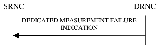
Figure 24: Dedicated Measurement Failure procedure, Successful Operation
