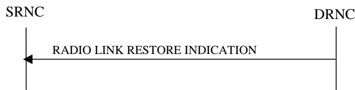
Figure 19: Radio Link Restoration procedure, Successful Operation
