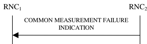
Figure 30E: Common Measurement Failure procedure, Successful Operation
