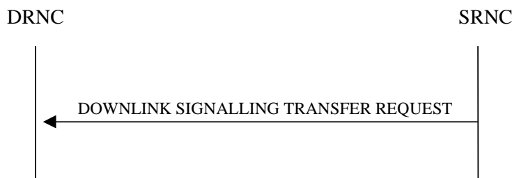
Figure 2: Downlink Signalling Transfer procedure, Successful Operation
