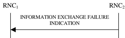
Figure 30J: Information Exchange Failure procedure, Successful Operation
