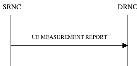
Figure 26H: UE Measurement Reporting procedure, Successful Operation
