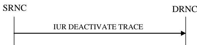
Figure 26L: Iur Deactivate Trace procedure, Successful Operation
