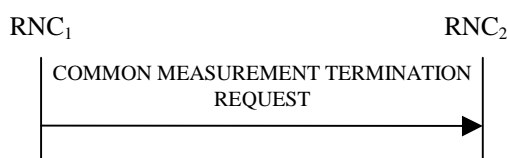
Figure 30D: Common Measurement Termination procedure, Successful Operation
