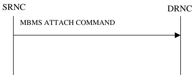
Figure 31: MBMS Attach procedure, Successful Operation
