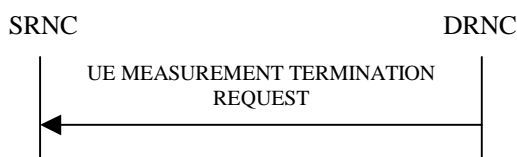
Figure 26I: UE Measurement Termination procedure, Successful Operation
