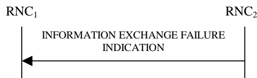
Figure 30J: Information Exchange Failure procedure, Successful Operation
