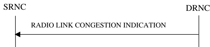
Figure 26C: Radio Link Congestion procedure, Successful Operation
