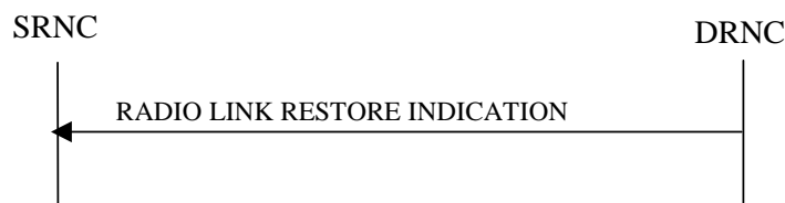
Figure 19: Radio Link Restoration procedure, Successful Operation
