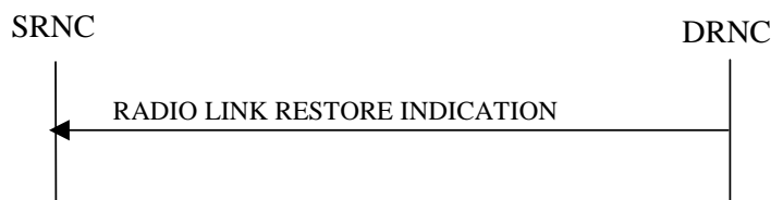
Figure 19: Radio Link Restoration procedure, Successful Operation
