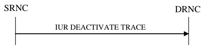
Figure 26L: Iur Deactivate Trace procedure, Successful Operation
