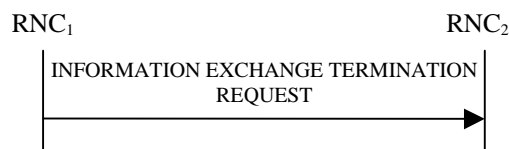
Figure 30I: Information Exchange Termination procedure, Successful Operation
