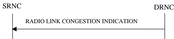
Figure 26C: Radio Link Congestion procedure, Successful Operation
