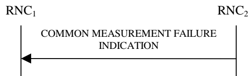
Figure 30E: Common Measurement Failure procedure, Successful Operation
