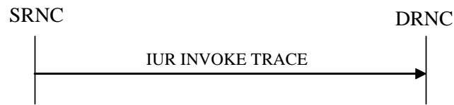
Figure 26K: Iur Invoke Trace procedure, Successful Operation
