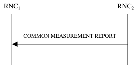
Figure 30C: Common Measurement Reporting procedure, Successful Operation
