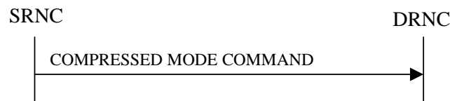
Figure 26: Compressed Mode Command procedure, Successful Operation
