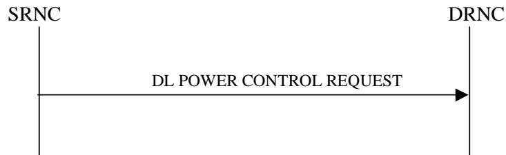
Figure 25: Downlink Power Control procedure, Successful Operation
