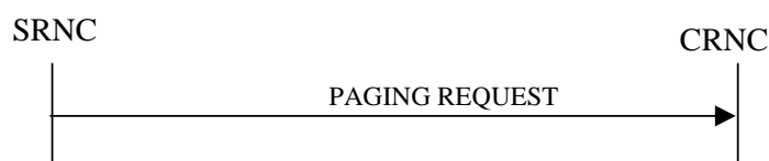
Figure 4: Paging procedure, Successful Operation
