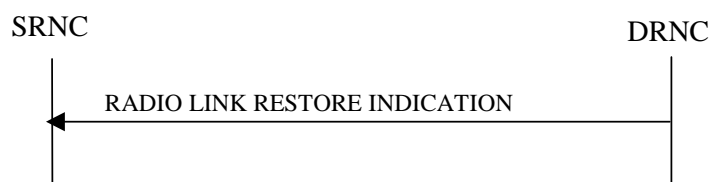
Figure 19: Radio Link Restoration procedure, Successful Operation
