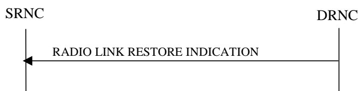
Figure 19: Radio Link Restoration procedure, Successful Operation
