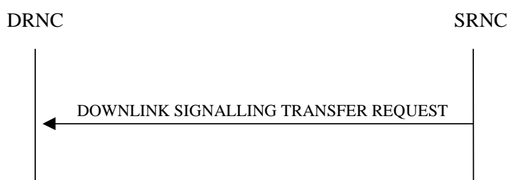
Figure 2: Downlink Signalling Transfer procedure, Successful Operation
