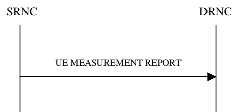
Figure 26H: UE Measurement Reporting procedure, Successful Operation
