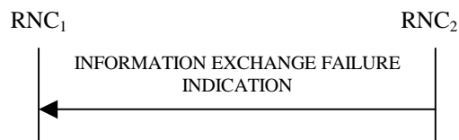
Figure 30J: Information Exchange Failure procedure, Successful Operation
