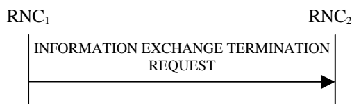
Figure 30I: Information Exchange Termination procedure, Successful Operation
