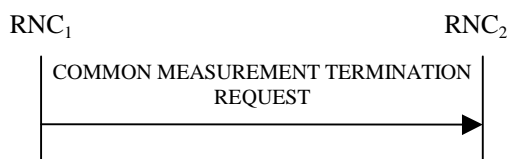
Figure 30D: Common Measurement Termination procedure, Successful Operation
