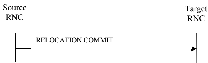
Figure 3: Relocation Commit procedure, Successful Operation
