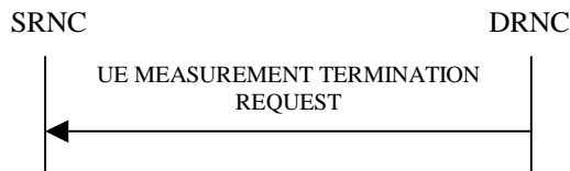
Figure 26I: UE Measurement Termination procedure, Successful Operation
