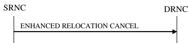
Figure 26O: Enhanced Relocation Cancel procedure: Successful Operation
