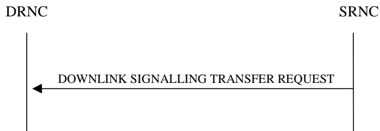
Figure 2: Downlink Signalling Transfer procedure, Successful Operation
