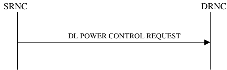
Figure 25: Downlink Power Control procedure, Successful Operation
