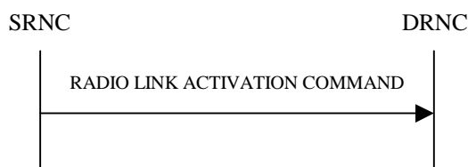
Figure 26D: Radio Link Activation procedure
