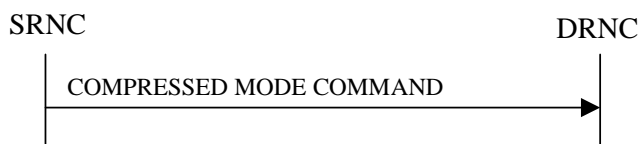
Figure 26: Compressed Mode Command procedure, Successful Operation
