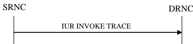
Figure 26K: Iur Invoke Trace procedure, Successful Operation
