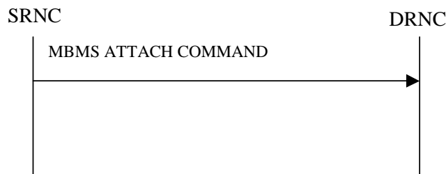
Figure 31: MBMS Attach procedure, Successful Operation
