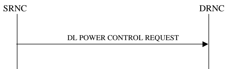
Figure 25: Downlink Power Control procedure, Successful Operation
