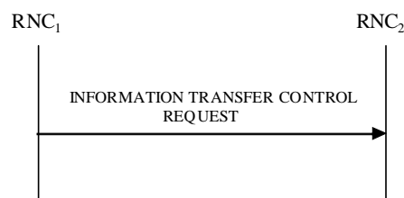
Figure 30M: Information Transfer Control procedure, Successful Operation
