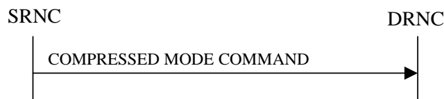
Figure 26: Compressed Mode Command procedure, Successful Operation
