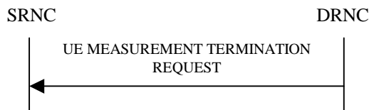
Figure 26I: UE Measurement Termination procedure, Successful Operation
