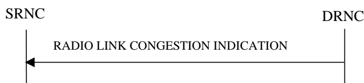
Figure 26C: Radio Link Congestion procedure, Successful Operation
