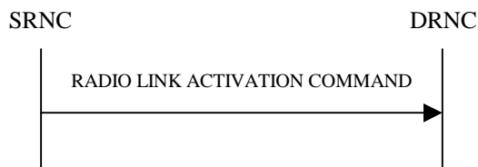
Figure 26D: Radio Link Activation procedure
