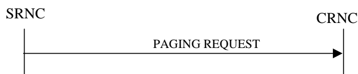
Figure 4: Paging procedure, Successful Operation
