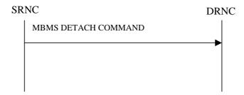
Figure 32: MBMS Detach procedure, Successful Operation
