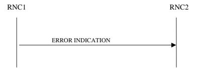
Figure 30: Error Indication procedure, Successful Operation
