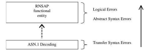
Figure 34: Protocol Errors in RNSAP
