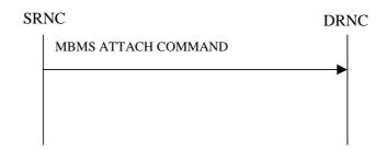
Figure 31: MBMS Attach procedure, Successful Operation
