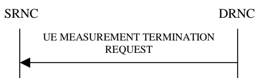
Figure 261: UE Measurement Termination procedure, Successful Operation
