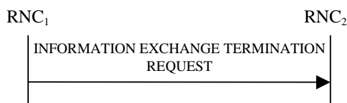
Figure 30I: Information Exchange Termination procedure, Successful Operation
