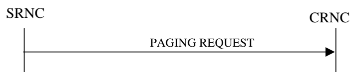
Figure 4: Paging procedure, Successful Operation
