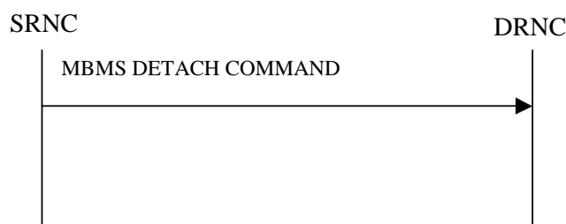
Figure 32: MBMS Detach procedure, Successful Operation
