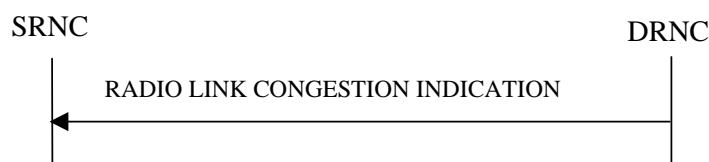
Figure 26C: Radio Link Congestion procedure, Successful Operation
