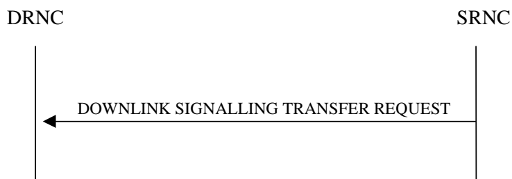
Figure 2: Downlink Signalling Transfer procedure, Successful Operation
