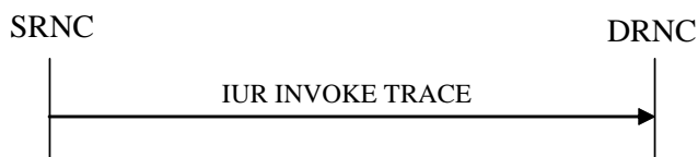
Figure 26K: Iur Invoke Trace procedure, Successful Operation
