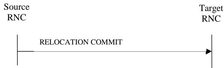
Figure 3: Relocation Commit procedure, Successful Operation
