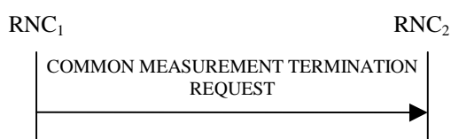
Figure 30D: Common Measurement Termination procedure, Successful Operation
