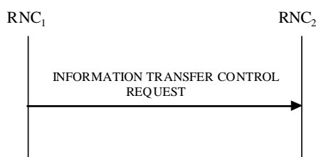
Figure 30M: Information Transfer Control procedure, Successful Operation
