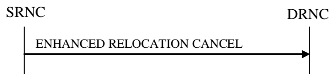
Figure 260: Enhanced Relocation Cancel procedure: Successful Operation
