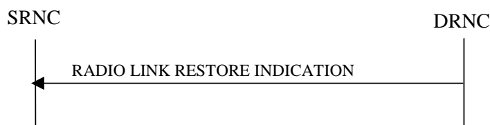
Figure 19: Radio Link Restoration procedure, Successful Operation
