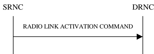
Figure 26D: Radio Link Activation procedure
