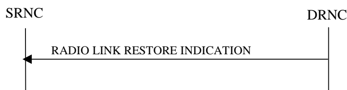
Figure 19: Radio Link Restoration procedure, Successful Operation
