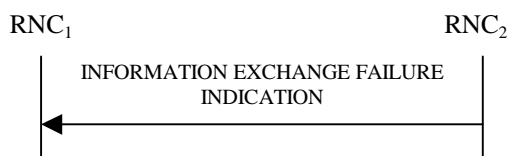
Figure 30J: Information Exchange Failure procedure, Successful Operation
