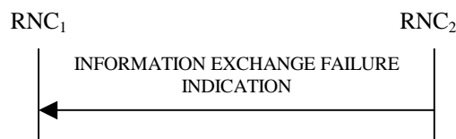
Figure 30J: Information Exchange Failure procedure, Successful Operation
