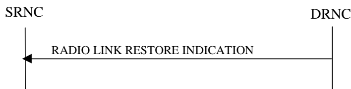
Figure 19: Radio Link Restoration procedure, Successful Operation
