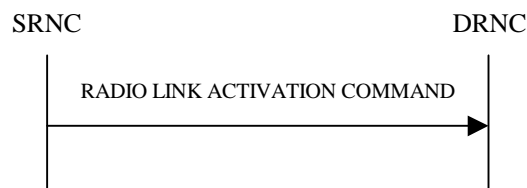
Figure 26D: Radio Link Activation procedure
