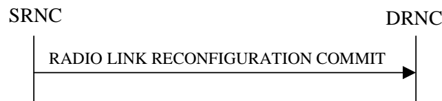
Figure 12: Synchronised Radio Link Reconfiguration Commit procedure, Successful Operation
