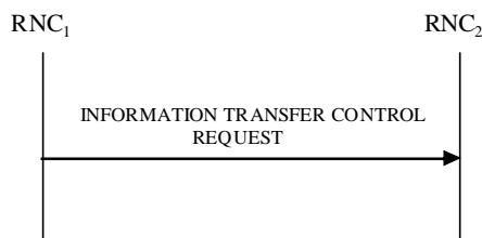
Figure 30M: Information Transfer Control procedure, Successful Operation
