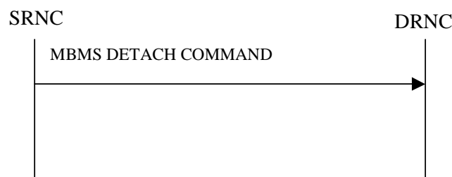
Figure 32: MBMS Detach procedure, Successful Operation
