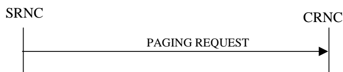
Figure 4: Paging procedure, Successful Operation
