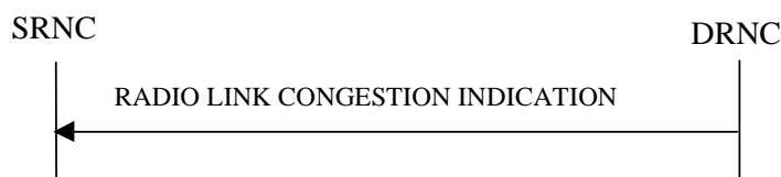
Figure 26C: Radio Link Congestion procedure, Successful Operation
