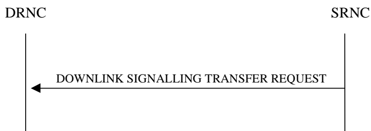
Figure 2: Downlink Signalling Transfer procedure, Successful Operation
