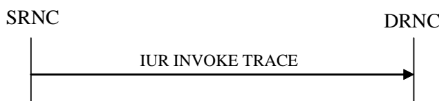
Figure 26K: Iur Invoke Trace procedure, Successful Operation
