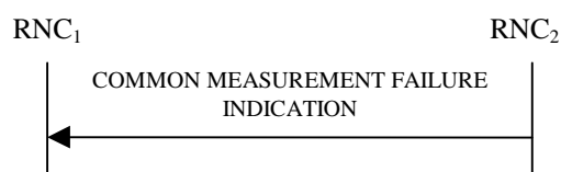
Figure 30E: Common Measurement Failure procedure, Successful Operation
