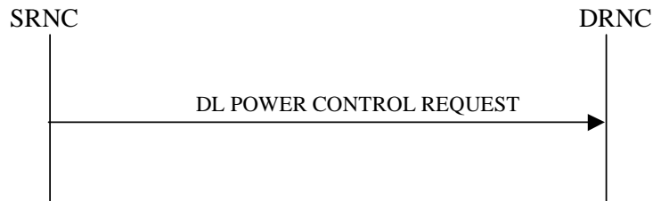
Figure 25: Downlink Power Control procedure, Successful Operation
