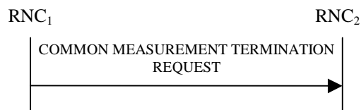
Figure 30D: Common Measurement Termination procedure, Successful Operation
