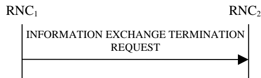
Figure 30I: Information Exchange Termination procedure, Successful Operation
