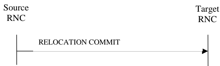
Figure 3: Relocation Commit procedure, Successful Operation
