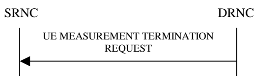
Figure 26I: UE Measurement Termination procedure, Successful Operation
