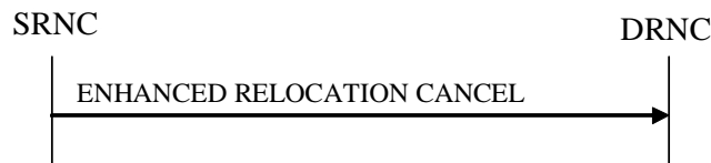
Figure 26O: Enhanced Relocation Cancel procedure: Successful Operation
