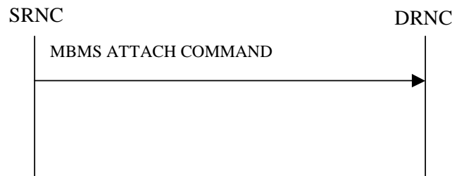
Figure 31: MBMS Attach procedure, Successful Operation
