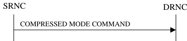
Figure 26: Compressed Mode Command procedure, Successful Operation
