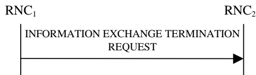
Figure 30I: Information Exchange Termination procedure, Successful Operation
