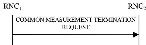
Figure 30D: Common Measurement Termination procedure, Successful Operation
