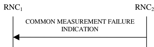
Figure 30E: Common Measurement Failure procedure, Successful Operation
