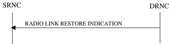
Figure 19: Radio Link Restoration procedure, Successful Operation
