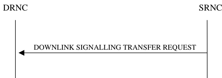
Figure 2: Downlink Signalling Transfer procedure, Successful Operation
