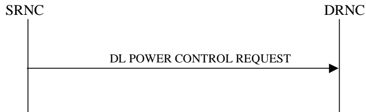
Figure 25: Downlink Power Control procedure, Successful Operation
