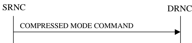
Figure 26: Compressed Mode Command procedure, Successful Operation
