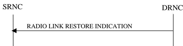
Figure 19: Radio Link Restoration procedure, Successful Operation
