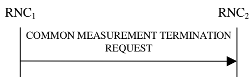
Figure 30D: Common Measurement Termination procedure, Successful Operation
