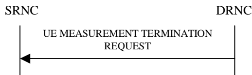
Figure 26I: UE Measurement Termination procedure, Successful Operation
