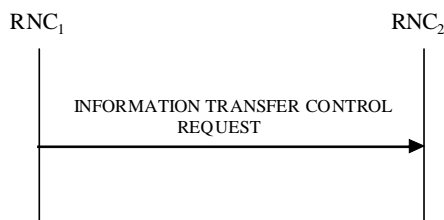
Figure 30M: Information Transfer Control procedure, Successful Operation
