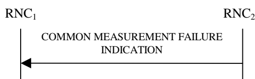
Figure 30E: Common Measurement Failure procedure, Successful Operation
