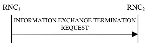
Figure 30I: Information Exchange Termination procedure, Successful Operation
