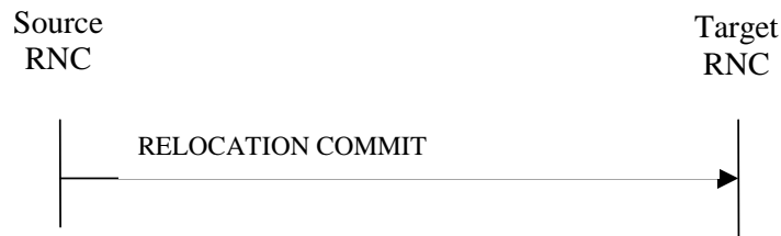
Figure 3: Relocation Commit procedure, Successful Operation
