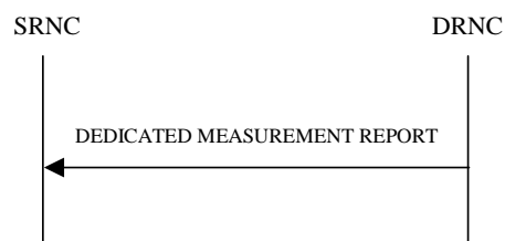
Figure 22: Dedicated Measurement Reporting procedure, Successful Operation
