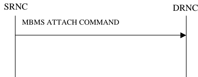
Figure 31: MBMS Attach procedure, Successful Operation
