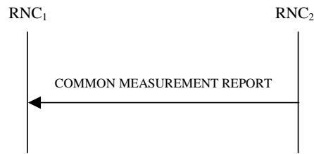
Figure 30C: Common Measurement Reporting procedure, Successful Operation
