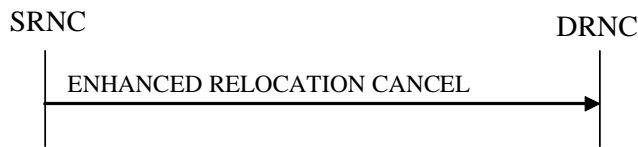
Figure 26O: Enhanced Relocation Cancel procedure: Successful Operation
