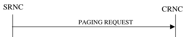
Figure 4: Paging procedure, Successful Operation
