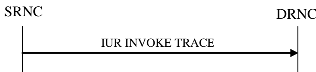
Figure 26K: Iur Invoke Trace procedure, Successful Operation
