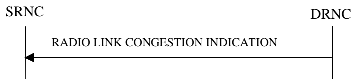
Figure 26C: Radio Link Congestion procedure, Successful Operation
