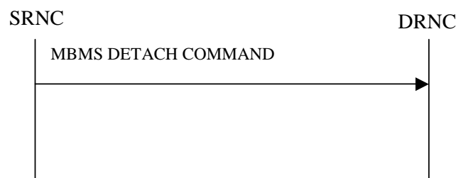
Figure 32: MBMS Detach procedure, Successful Operation
