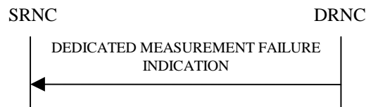
Figure 24: Dedicated Measurement Failure procedure, Successful Operation
