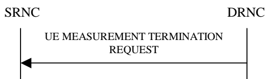
Figure 26I: UE Measurement Termination procedure, Successful Operation
