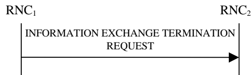
Figure 30I: Information Exchange Termination procedure, Successful Operation
