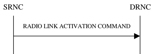
Figure 26D: Radio Link Activation procedure
