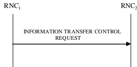
Figure 30M: Information Transfer Control procedure, Successful Operation
