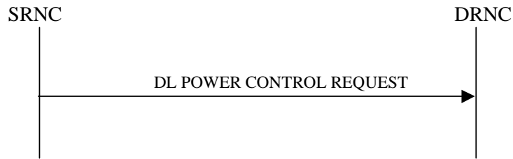
Figure 25: Downlink Power Control procedure, Successful Operation
