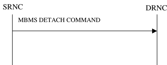
Figure 32: MBMS Detach procedure, Successful Operation
