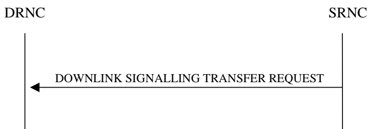
Figure 2: Downlink Signalling Transfer procedure, Successful Operation
