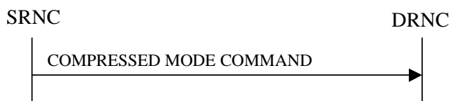
Figure 26: Compressed Mode Command procedure, Successful Operation
