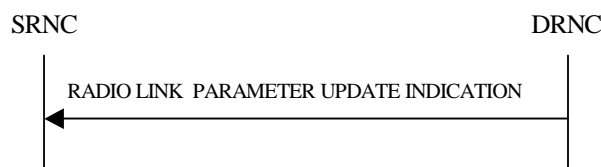
Figure 26E: Radio Link Parameter Update Indication, Successful Operation
