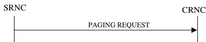
Figure 4: Paging procedure, Successful Operation
