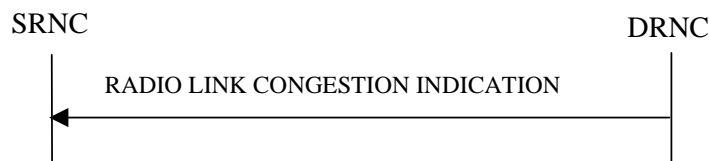
Figure 26C: Radio Link Congestion procedure, Successful Operation
