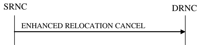
Figure 26O: Enhanced Relocation Cancel procedure: Successful Operation
