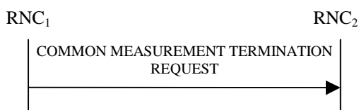
Figure 30D: Common Measurement Termination procedure, Successful Operation
