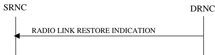
Figure 19: Radio Link Restoration procedure, Successful Operation
