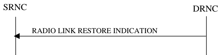
Figure 19: Radio Link Restoration procedure, Successful Operation
