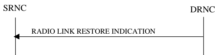
Figure 19: Radio Link Restoration procedure, Successful Operation
