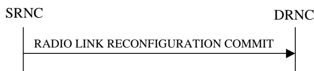
Figure 12: Synchronised Radio Link Reconfiguration Commit procedure, Successful Operation–[FDD - If the Activation Delay IE is included in the RADIO LINK RECONFIGURATION COMMIT message, the DRNS shall if supported send the HS-SCCH order to execute the TTI switching process according to TS 25.214 [10]. The CFN IE in the RADIO LINK RECONFIGURATION COMMIT message shall be ignored by the DRNS.]
