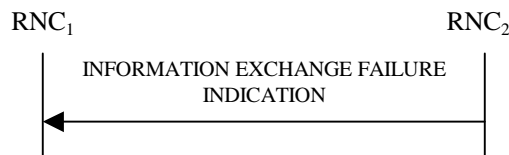
Figure 30J: Information Exchange Failure procedure, Successful Operation
