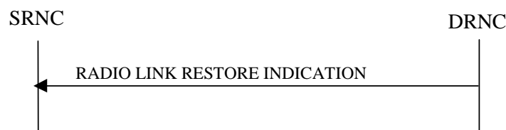
Figure 19: Radio Link Restoration procedure, Successful Operation
